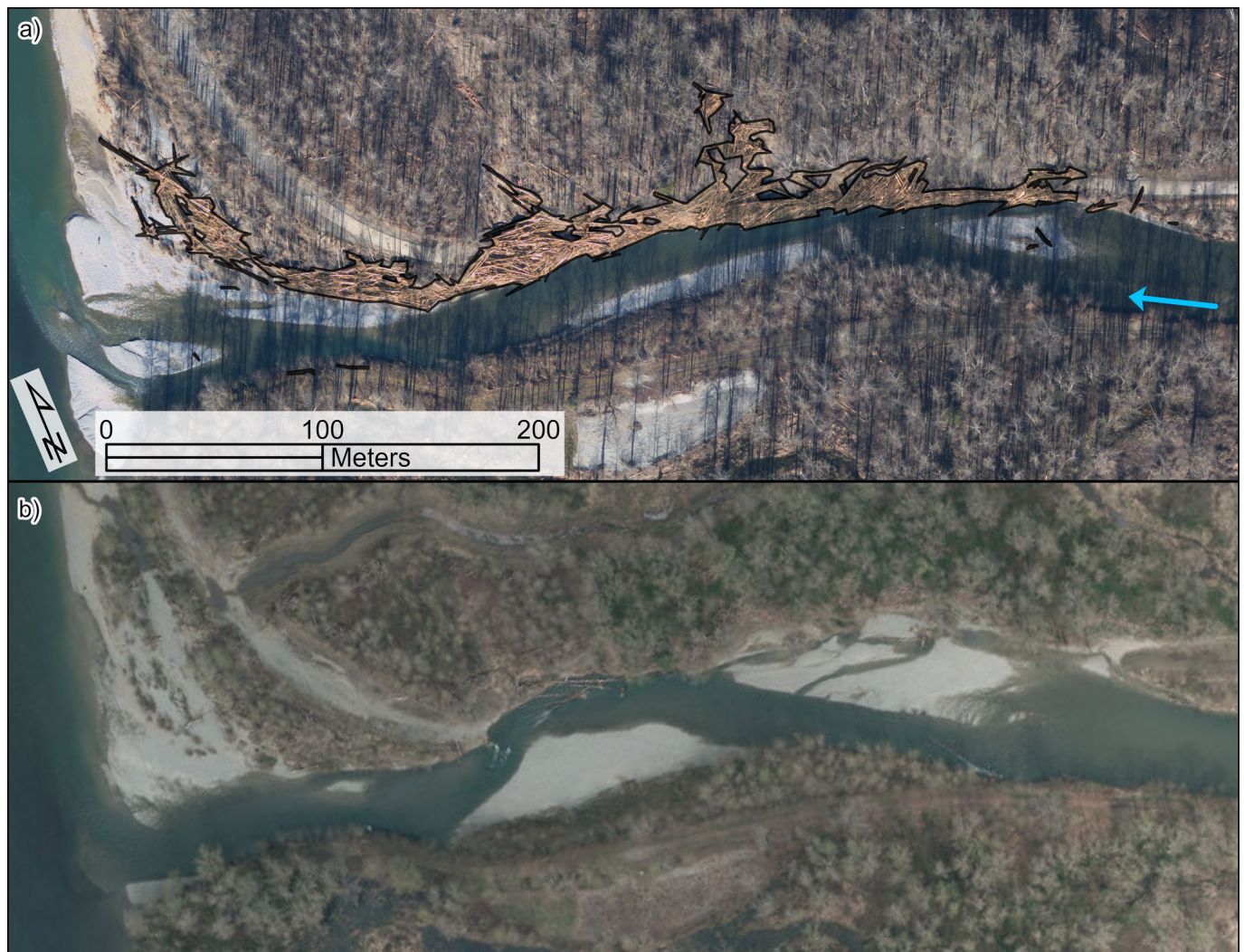
Figure 10 2009 aerial image showing the extent (highlighted in orange with black outline) of the wood raft that formed at the Tolt-Snoqualmie confluence following the January 2009 flood (a) and the same area in 2012 (b). Blue arrow indicates flow direction.
