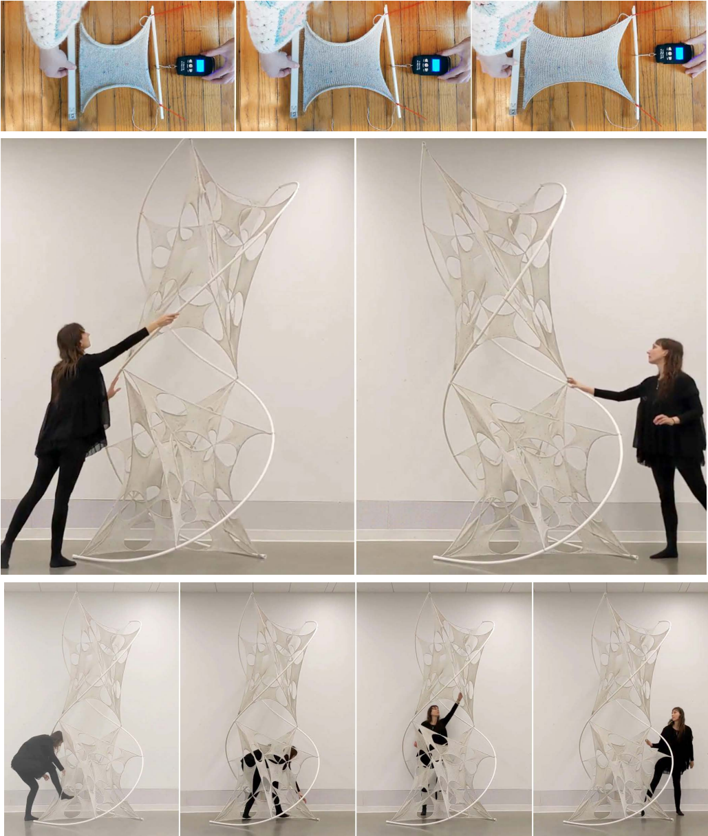
Figure 2. Studying elastic properties of knit material samples with a spring scale. Photo Credit: Virginia Melnyk.
