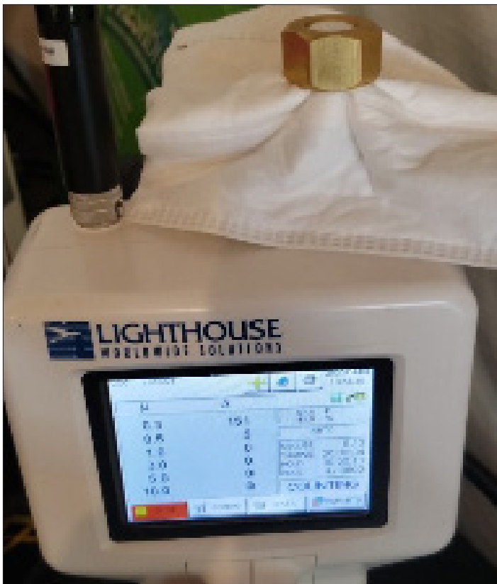
Figure 3. Measuring MERV 15 material capacity in room at 0.1 CFM.
