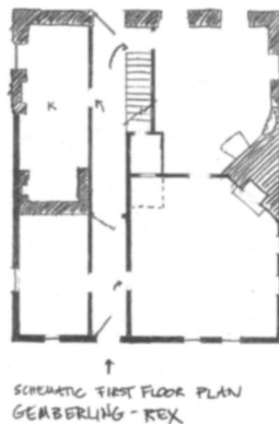
Figure 14: Schematic plan, period III, showing the narrow, non-classical center passage, rear-facing stairs, and two large parlors. By the author.
