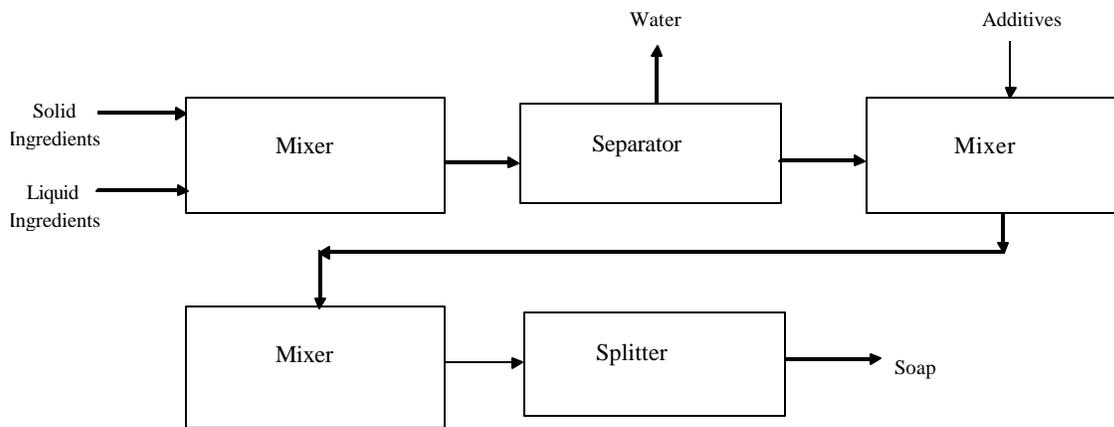
**Figure 3: Block Flow Diagram for Soap Manufacturing**
