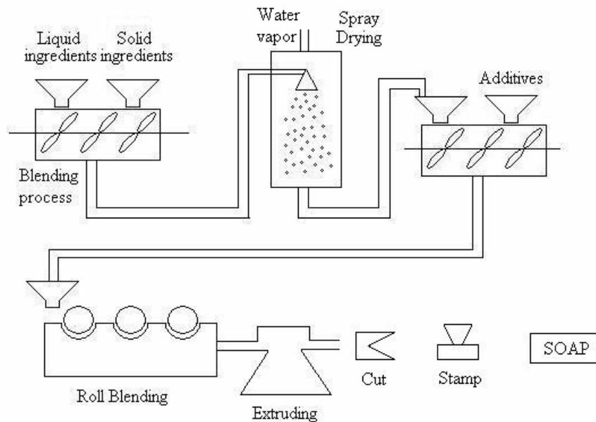
**Figure 1: Process for the Manufacture of Soap**
