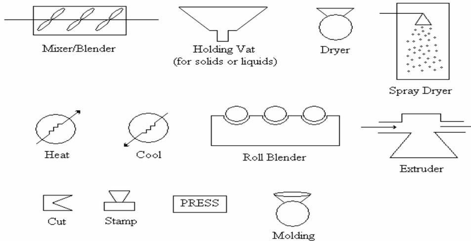
**Figure 2: Process Symbols for Unit Operations**
