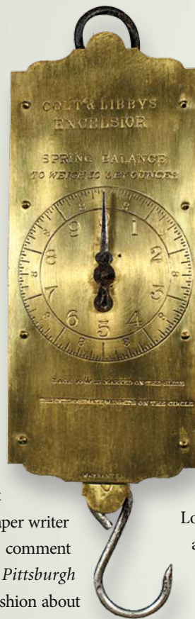
This brass and steel spring balance scale was one of at least a dozen found on the Arabia .
