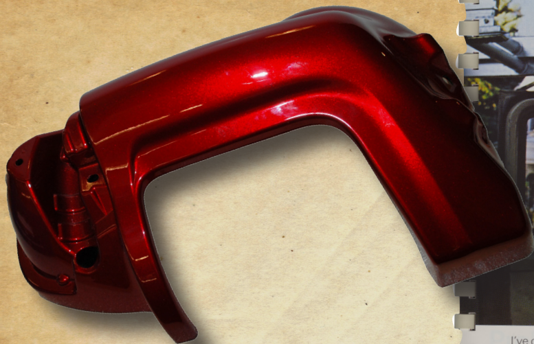
Above: Vehicle part with PPG Andaro HC coating, 2008. The coating has high clarity of color while also being highly fade-resistant.
